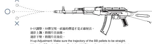
When the BB pellet flies up: Push the H-UP lever forward to lower the trajectory. When the BB pellet falls down: Push the H-UP lever backward to raise the trajectory.
