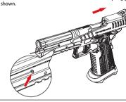
⑤ Push the Slide backward and align the notch corresponds to the slide stop as shown.
