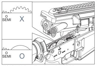
3號齒在槍身結合時,必須轉到正確位置,才可將上槍身蓋下。 Make sure the sector gear is turned to the correct position before reassembling the receiver / gearbox.
