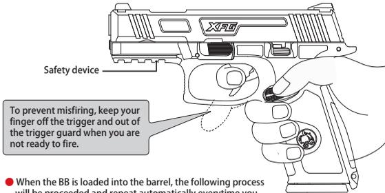
When the BB is loaded into the barrel, the following process will be proceeded and repeat automatically everytime you pull the trigger: BB fired → Slide movement (blowed backward) → Load the next BB (slide re-positioned)
