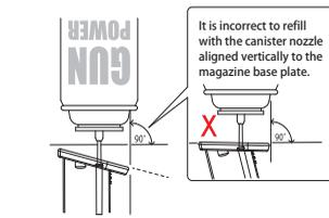
Please turn the magazine up side down to keep the injection hole side up, fill the gas only when the canister is verticalized to the injection hole. The gas will not be filled into the magazine or will leak out if the canister is not verticalized to the injection hole.
