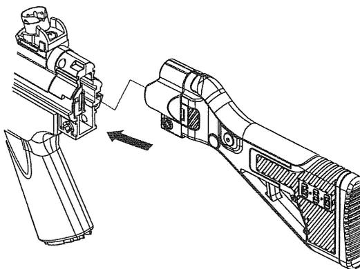
**3** Insert the pin to finish installation
