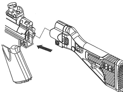
**3** Insert the pin to finish installation
