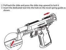
⑤ Press the slide stop button on the right to remove it. Push the slide forward to detach it. Meanwhile. The recoil spring The recoil spring guide set can be easily removed by slightly Push the outer barrel set forward to remove. You may disassemble the recoil spring guide by detaching the dedicated tool if necessary. Please keep your finger off the trigger and
