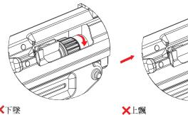
★下墜 Rotate the dial clockwise to make the pellet go up
