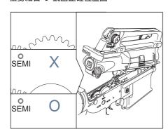
3號齒在槍身結合時,必須轉到正確位置: 才可將上槍身蓋下。Make sure No.3 gear is turned to the correct position before you reassemble the receiver/gearbox.
