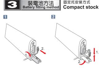
將槍托底板蓋打開再拉出電線 Lower the buttplate latch with your fingernail and open the cover. Pull out the connector.
